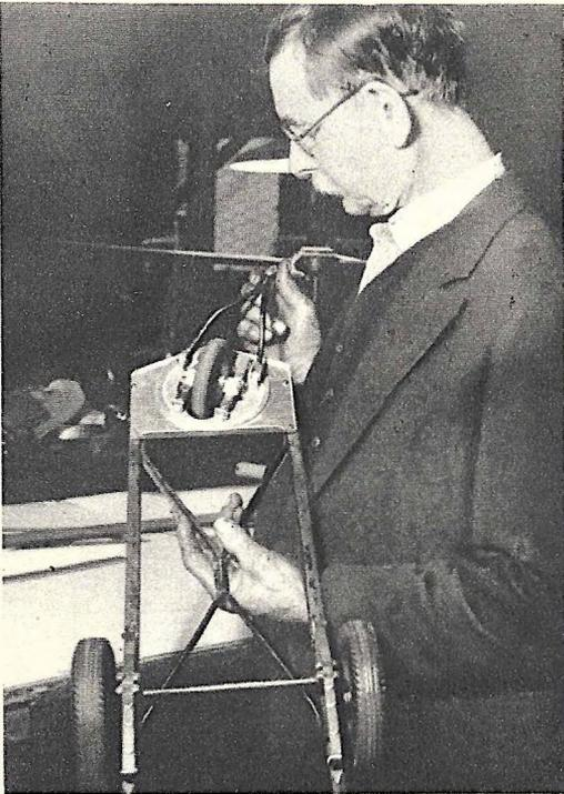
A third wheel shown in model is designed to remove weight from towing car and to end rear spring and axle breakdown. Device eases riding by removing much swaying and bobbing.
