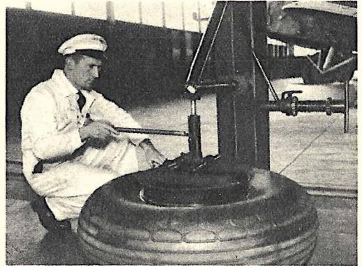
United Air Lines mechanic demonstrates device developed for quick and easy removal of tires from air liners. Jack and auto rim device loosens and forces tire from airplane wheel.
