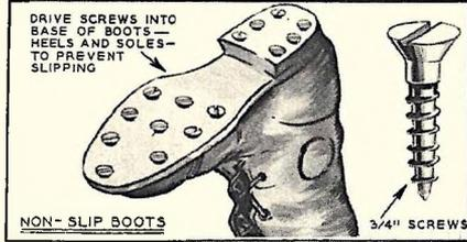
The drawing shows special construction for boot soles to prevent slipping on dangerous rocky stream beds.
