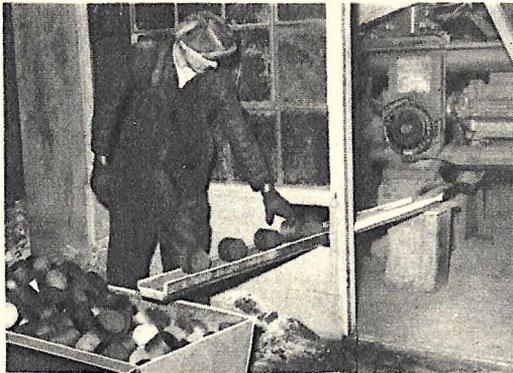
Frank Petrovick, foundryman, examines eight-pound scrap metal briquettes used for making castings. Briquettes are formed under 350-ton pressure. (Milwaukee Journal Photo)
