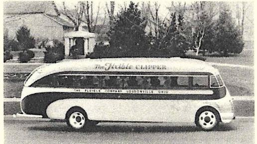
"The Flexible Clipper," ultra-streamlined bus, carries 20 passengers, and is powered by 78 h. p. engine. With safety glass throughout, de luxe chairs and down pillows are provided.
