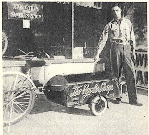
Designed for camping or delivery use, this midget bicycle trailer built by William Moll, of Minneapolis, Minn., has a built-in radio controlled from the bicycle's handlebars.
