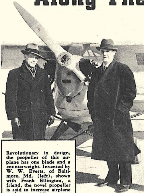
Revolutionary in design, the propeller of this airplane has one blade and a counterweight. Invented by W. W. Everts, of Baltimore, Md. (left), shown with Frank Ellington, a friend, the novel propeller is said to increase airplane performance 25 per cent.
